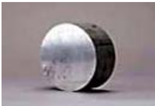
Starting with a solid billet of material (Aluminum or Magnesium alloy)
