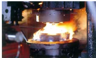
The next forging establishes the spoke shape and thickness
